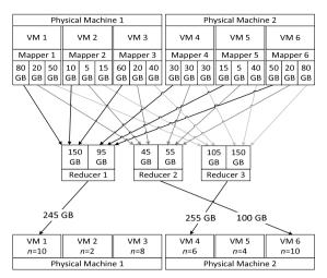
Fig. 6. Virtual machine mapper.
