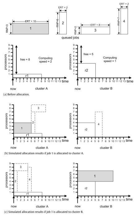
Fig. 4. Illustration of how TLA works.
