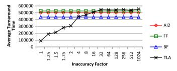
Fig. 8. Effect of inaccuracy in job runtime estimation.
