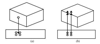
Fig. 1. (a) A changed voxel is projected onto the image plane. (b) The pixels surrounding the projected point must be updated.
