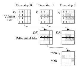
Fig. 3. An example of extracting the differential files and SOD. Grey parts represent changed voxels.
