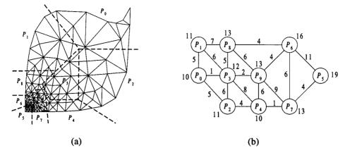
*Figure 2.* An example of a processor graph. (a) A partition of an irregular finite element graph. (b) The corresponding processor graph obtained from (a).
