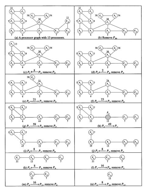
*Figure 3.* A step by step determination of the load transfer sequence by using the dynamic diffusion heuristic for the processor graph shown in (a).
