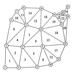
*Figure 1.* An example of a 21-node finite element graph with 24 finite elements (the circled and uncircled numbers denote the node numbers and finite element numbers, respectively).
