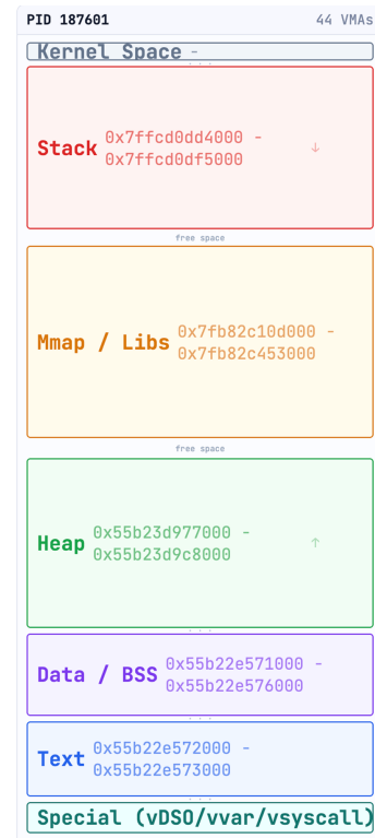
Fig. 13. Visualization of a single process's virtual address space.
