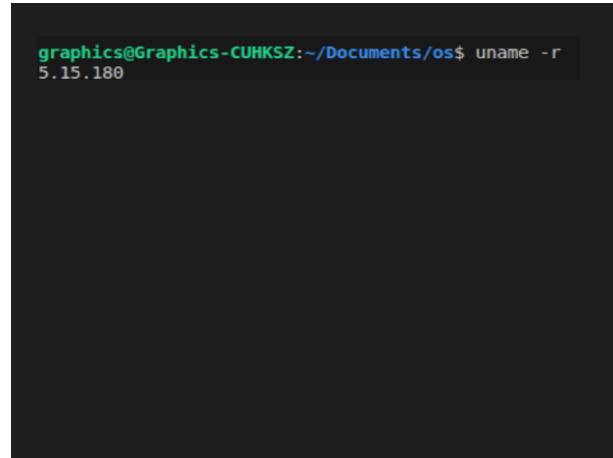
Fig. 1. Verification that the system booted into the modified Linux 5.15.180 kernel.
