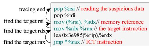
Fig. 12. Tracing memory reference.
