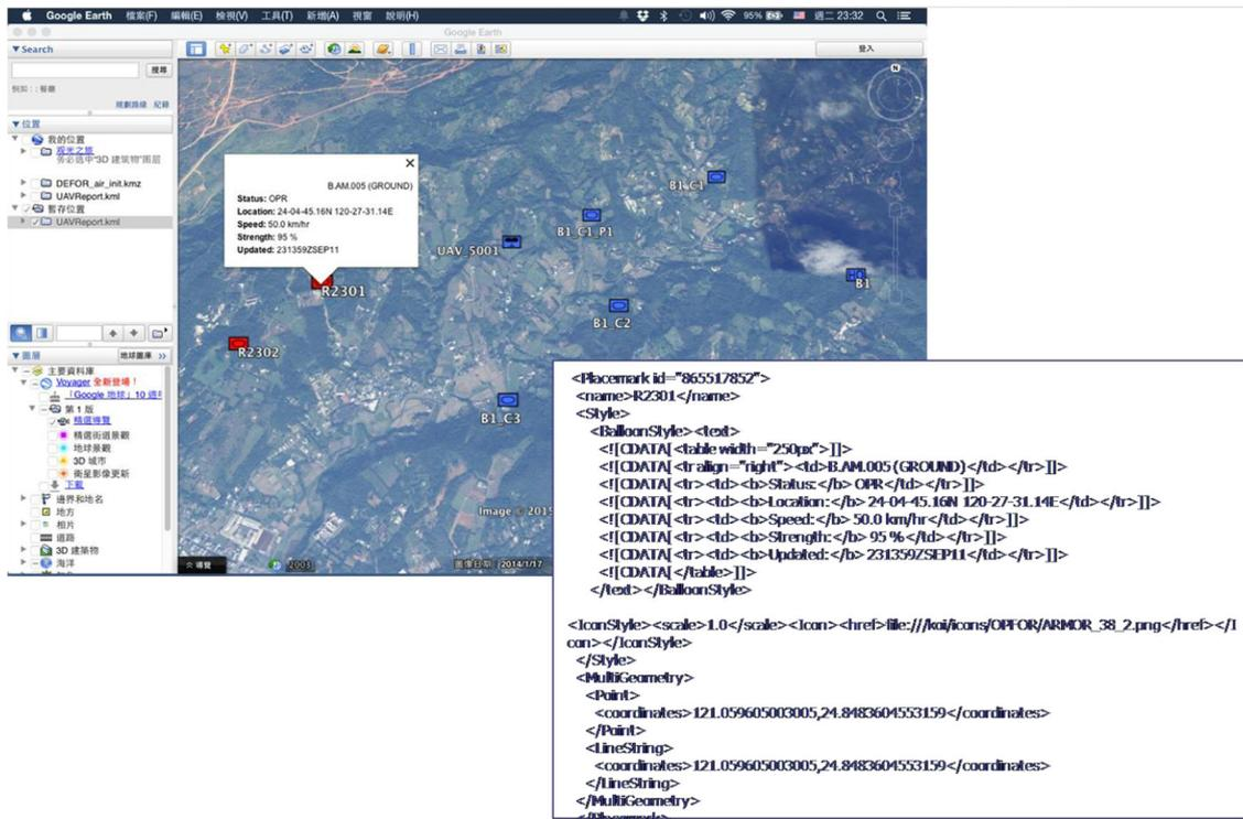
Fig. 13 Situation Display using Google Earth via KML data representation
