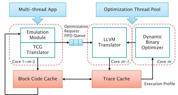
Fig. 1. Major components of HQEMU on an  $m$ -core platform.
