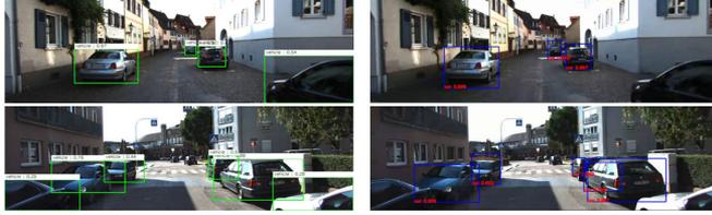
Fig. 8. KITTI detection result comparison: Left column: detection results of this work (ResNet-50); Right column: detection result of Faster R-CNN (VGG-16).
