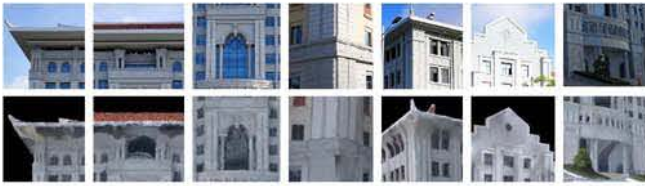
Figure 2: Matching cross-domain image patch pairs. Top: ground camera image patches; Bottom: UAV 3D model rendered image patches.
