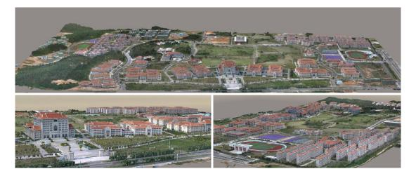
Figure 5. The generated 3D image-based point cloud of the Xiangan campus of Xiamen University.
