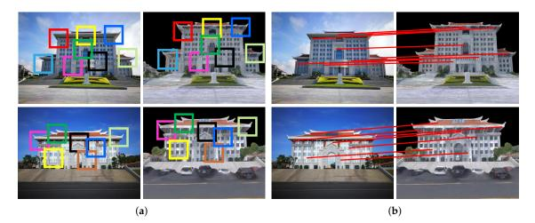
**Figure 14.** Cross-domain image patch matching results and center point connection of matching image patches. Left: Ground camera images; Right: Rendered images with the same viewpoint of ground camera image. (a) Cross-domain image patch matching results. (b) Center point connection of the matching image patches in (a).
