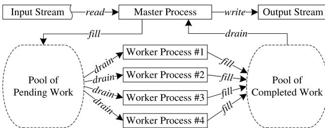
**Fig. 5** A master-worker streaming system
