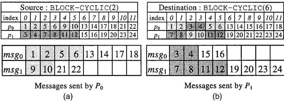
Figure 5. (a) A BLOCK-CYCLIC(2) to BLOCK-CYCLIC(6) redistribution on  $A[1:24]$  over  $M = 2$  processors. (b) Messages packed by source processors.
