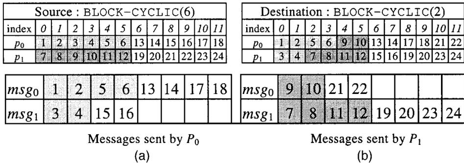
Figure 3. (a) A BLOCK-CYCLIC(6) to BLOCK-CYCLIC(2) redistribution on  $A[1:24]$  over  $M=2$  processors. (b) Messages packed by source processors.
