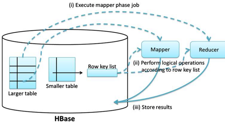
**Fig. 6** Implementation of CROSS JOIN
