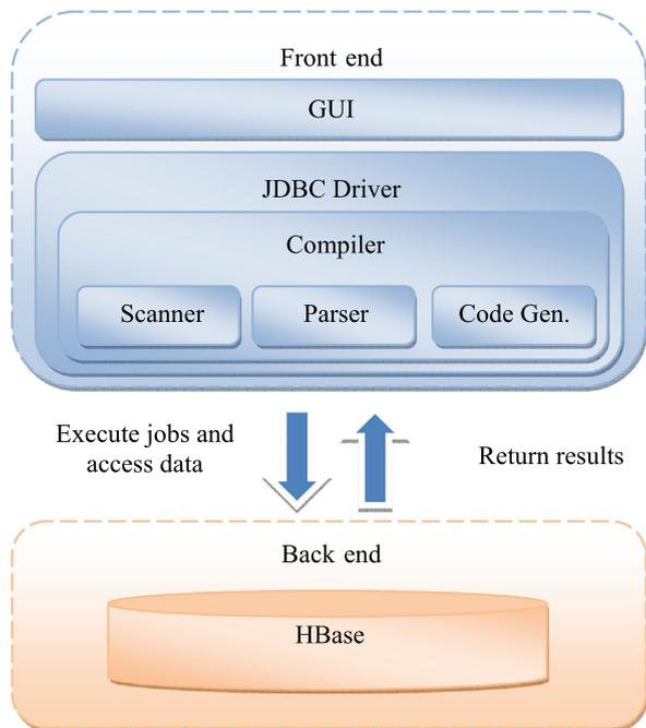
compiler to scan, parse and execute queries. The scanner, parser and code generator are implemented using the open source project, Druid. While an ANSI-SQL query submitted, the scanner breaks queries into tokens. The parser manipulates the abstract syntax tree which is comprised of tokens. The code generator produces MapReduce jobs to access HBase and then perform logical operations according to the parsed commands. The results of ANSI-SQL queries are returned and shown on GUI.
