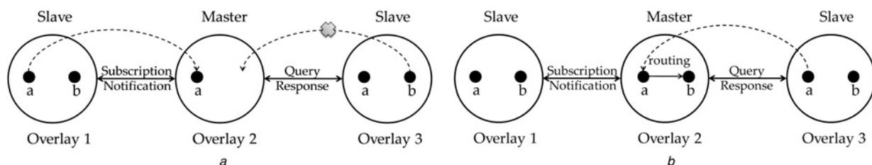
**Fig. 1** Two inter-overlay protocols in the master-slave model
