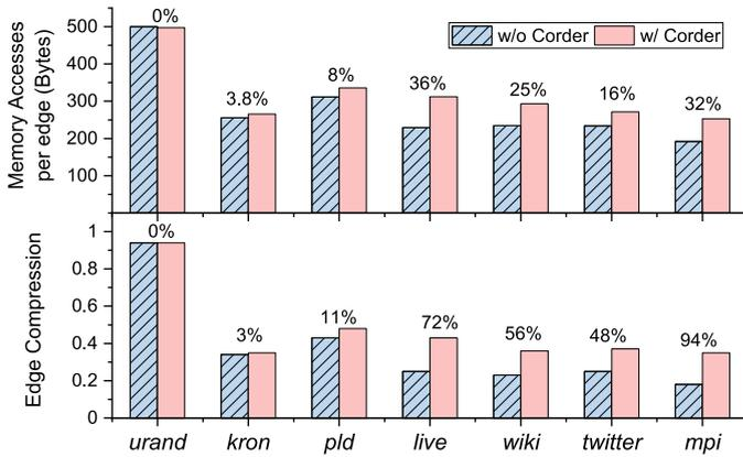
Fig. 8. Upper: Sustained memory bandwidth. Lower: No. of compressed edges compared to no. edges in the original graphs. Corder inflates graph inter-edges and thus raises memory traffic. Every pair of results (w/o versus w/ Corder) is denoted with the increased percentage.
