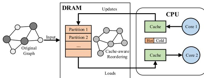
Fig. 3. Conceptual design of Corder. Grey cycles represent subgraphs. Different grey colors and sizes indicate imbalanced workloads. Corder reorders the graph such that the vertex subset of each subgraph can fit into the private caches of multicores with fairly balanced loads. Within the cache, hot vertices and cold ones are segmented to improve cache locality.
