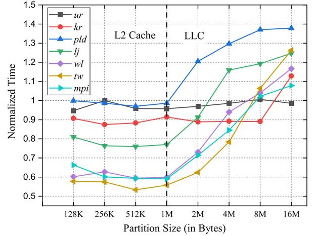
Fig. 10. The impact of partition size on the execution time. The time is normalized by the result of unordered graph.
