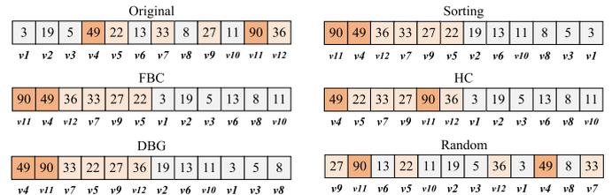
Fig. 2. Vertex placement by different reordering techniques. The degrees of vertices are filled inside the box. Cold vertices (degree  $\leq 20$ ) are painted with grey, hot vertices are colored, and very hot vertices (degree  $> 40$ ) are depicted with darker shade. Indexes below the box are the original vertex IDs.
