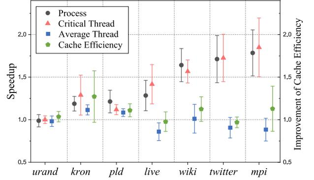
Fig. 7. The impact of Corder on thread behaviors and cache efficiency. The speedups (left) of graph processing, critical thread, and average thread are plotted with the improvement of cache efficiency (right). The results are calculated by the mean of different graph applications with 90 percent confidence interval.
