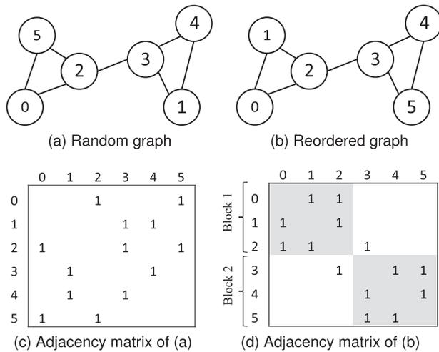
Fig. 1. Graphs and their belonging adjacency matrices. Graph (b) is reordered from graph (a) by assigning continuous ID numbers to neighboring vertices. The reordered vertices constitute two diagonal blocks, which are depicted with shadow color in matrix (d).
