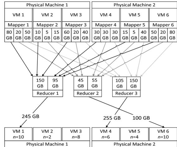
Fig. 6. Virtual machine mapper.
