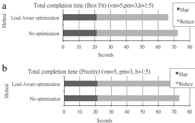
**Fig. 14.** Total completion time with load aware optimization: (a) Best fit method. (b) Priority method.
