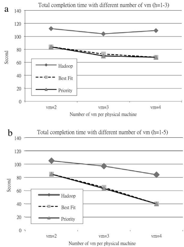
**Fig. 15.** Total completion time for different number of virtual machines. Using high heterogeneity, vm = 5.
