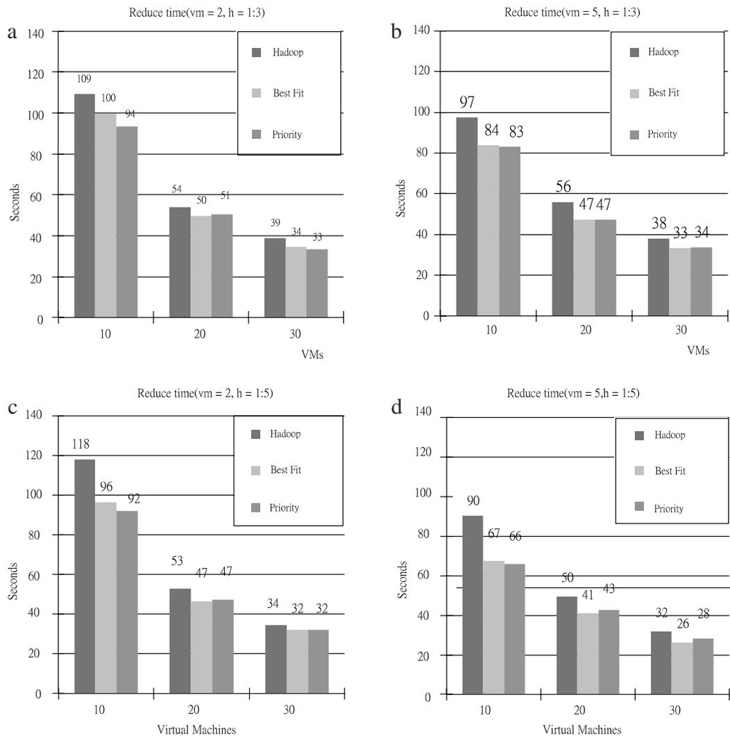
**Fig. 12.** Reduce completion time (a) low heterogeneity,  $vm = 2$ , (b) low heterogeneity,  $vm = 5$ , (c) high heterogeneity,  $vm = 2$ , (d) high heterogeneity,  $vm = 5$ .
