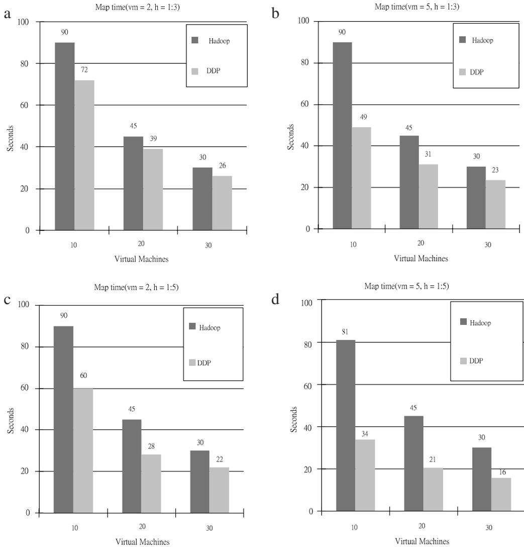
Fig. 11. Map completion time (a) low heterogeneity,  $vm = 2$ , (b) low heterogeneity,  $vm = 5$ , (c) high heterogeneity,  $vm = 2$ , (d) high heterogeneity,  $vm = 5$ .
