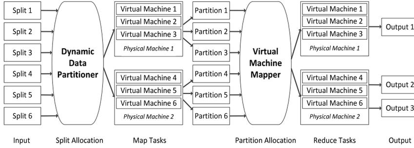
Fig. 3. Dataflow of dynamic data partitioner and virtual machine mapper.
