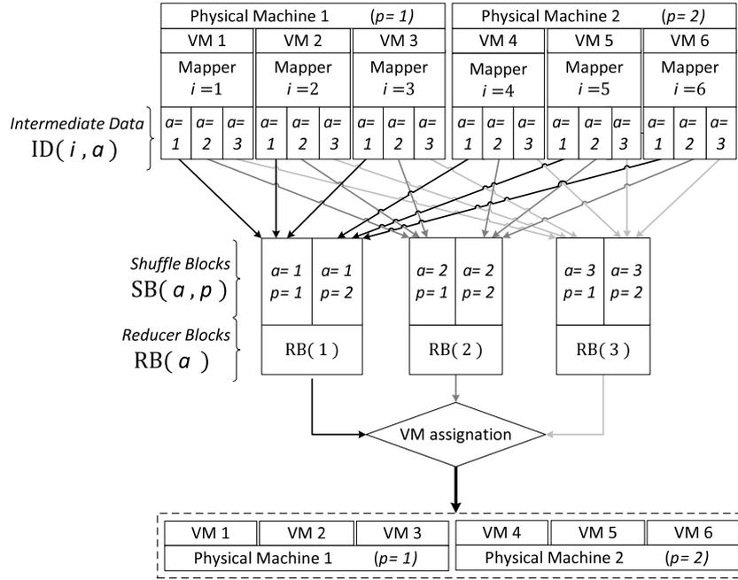
Fig. 5. Virtual machine mapper model.
