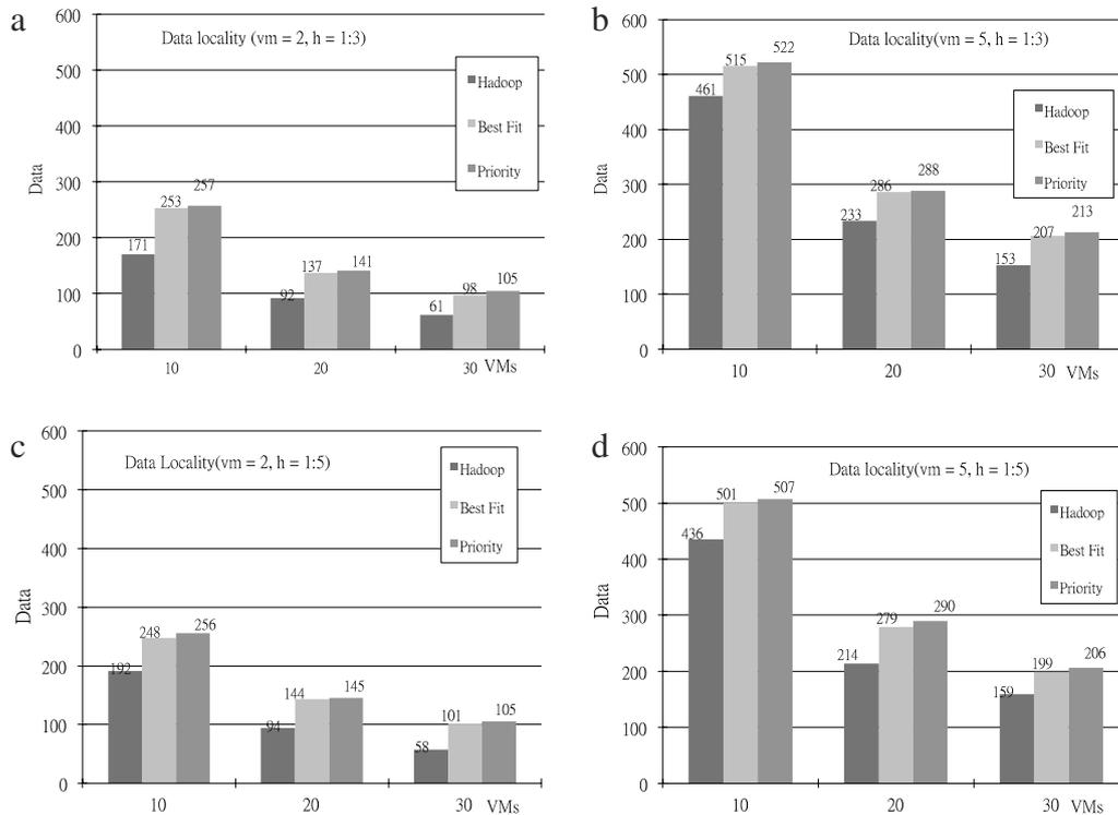
Fig. 10. Data locality (a) low heterogeneity,  $vm = 2$ , (b) low heterogeneity,  $vm = 5$ , (c) high heterogeneity,  $vm = 2$ , (d) high heterogeneity,  $vm = 5$ .
