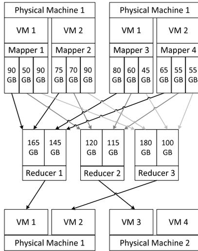
**Fig. 8.** VMM priority fit: reducers are assigned to a virtual machine based on data locality. Using a priority based order, Reducer 2 is reassigned to physical machine 2.
