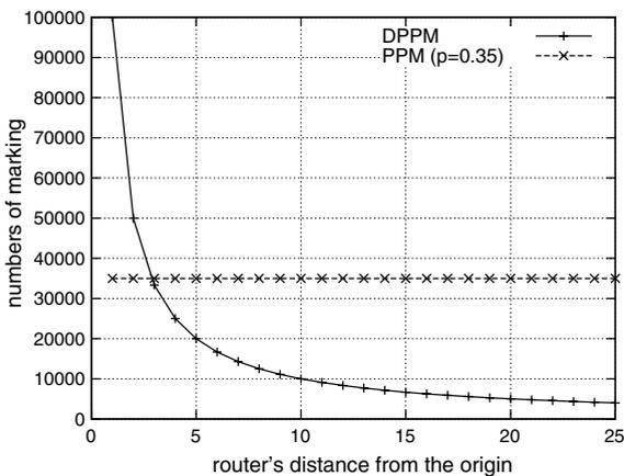
Fig. 5. A comparison of individual overheads.
