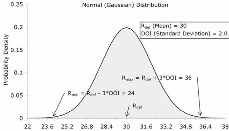
**Fig. 2.** The relationship between  $R_{def}$ ,  $R_{min}$ , and  $R_{max}$ .
