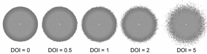
**Fig. 1.** The radio propagation range under different DOI.
