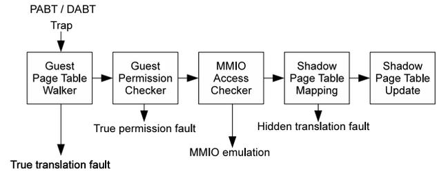
Figure 4: The emulation flow of shadow paging
