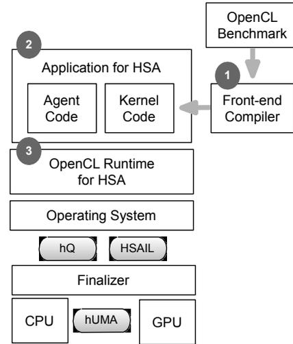
**Fig. 4. A basic HSA software stack tested by HSAemu.**
