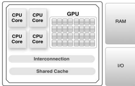
Fig. 1. Heterogeneous System Architecture.
