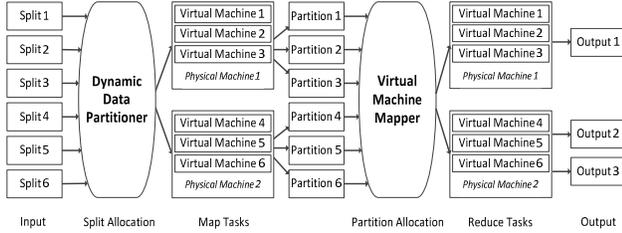
Figure 2. Dataflow of MapReduce model with the proposed dynamic data partitioner and a virtual machine mapper. Six Map tasks and three Reduce tasks run on virtual machines with differing processing capabilities.
