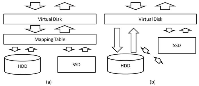
Fig. 1. The usage SSD in two scenario: Scenario (a) is the case which both SSD and HDD are combined into one virtual disk. The mapping table handle the re-direction of request. Scenario (b) is the case which SSD is the storage cache of HDD.
