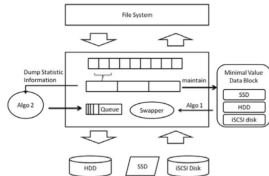
Fig. 3. The implementation of our heterogeneous storage system management mechanism.
