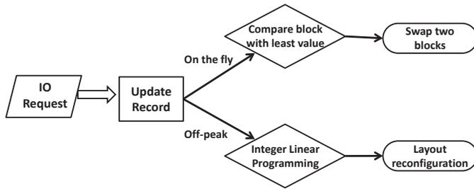
Fig. 2. The workflow of the trigger policy: When the new IO request coming, the system update the record and identify the request is hot or not. In the situation of on the fly, system only migration the block which value exceeds the threshold. In the situation of off-peak, the system will consider the full blocks and re-allocate into the suitable placement.
