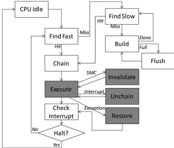
Figure 1. Typical flow of a full system emulator using dynamic binary translation.
