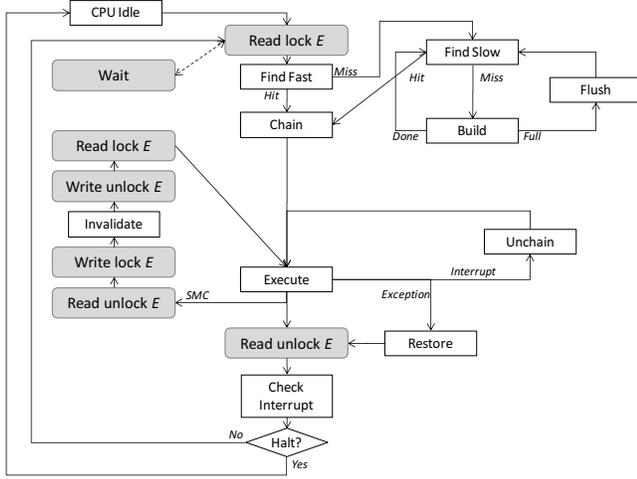
Figure 4. Modified emulation flow for PQEMU using SCC design. Due to sharing components duplication, only lock E exclusive\_rwlock is required, in comparison to UCC design.
