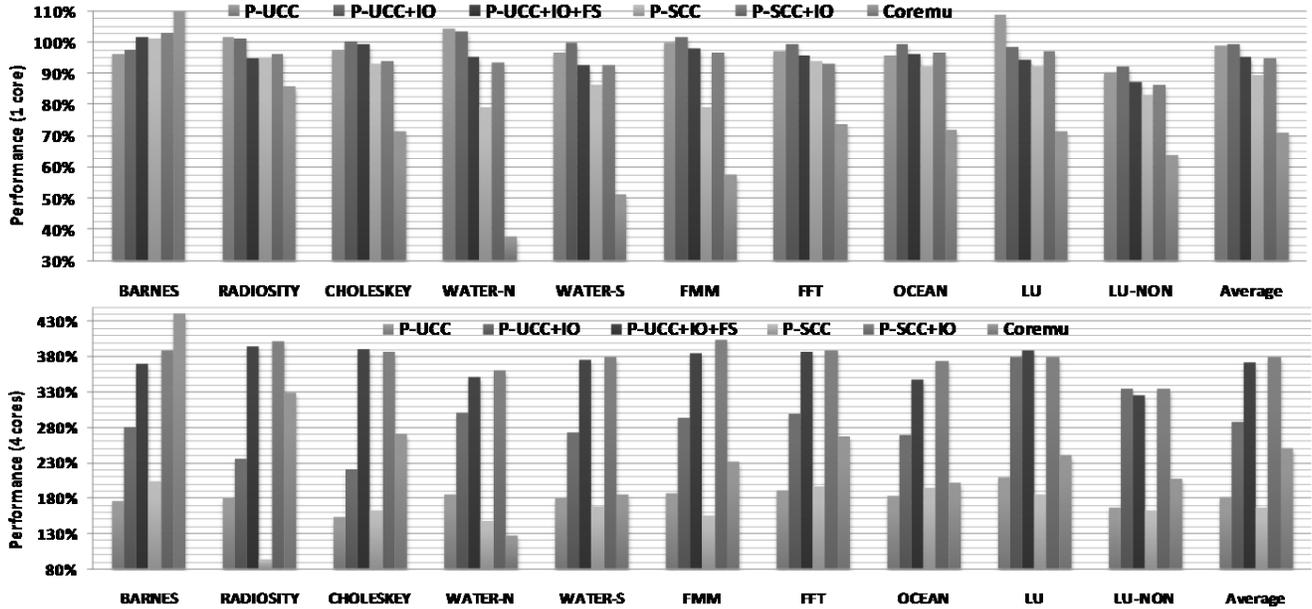
Figure 5. Performance by computation time of SPLASH-2 benchmarks using one (upper) and four (lower) working threads. We treat baseline QEMU as 100% basis.
