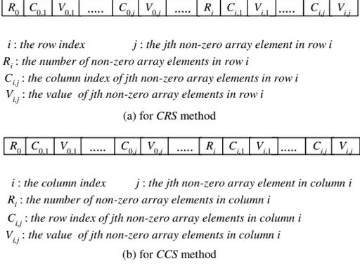
Figure 6: The formats of the special buffer B.
