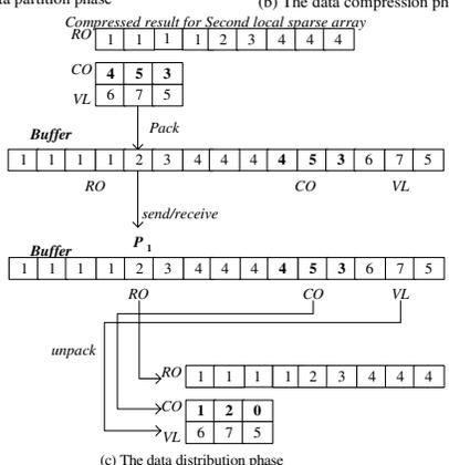
Figure 5: An example of the CFS scheme.
