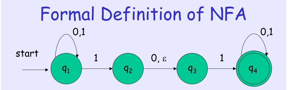
$Q = \{q_1, q_2, q_3, q_4\}, \qquad \Sigma = \{0, 1\}, \\ q_{start} = q_1, \qquad F = \{q_4\}, \end{cases}$
