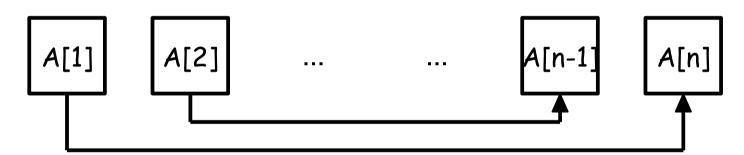
Running time = (n - 1) + (n - 2) + ... + 1=  $c_1 n^2 + c_2 n + c_3 = \Omega(n^2)$ ( $c_1, c_2$  and  $c_3$  are constants)
