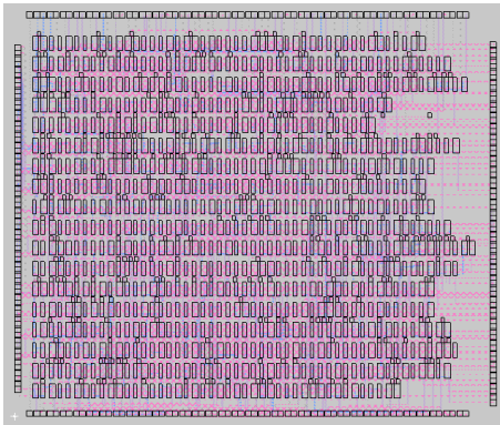
Fig. 12: Post place-and-route of dec circuit which is mapped by BM. Dimensions are 3960\mu\text{m} \times 3310\mu\text{m} . The dimensions are increased to 4870\mu\text{m} \times 3990\mu\text{m} when the circuit is mapped using the map command of ABC.
