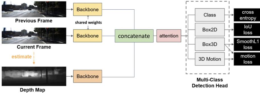
**Fig. 1.** The overall architecture of the proposed network that integrates 2D/3D object detection and 3D object motion estimation for multi-frame monocular images. The outputs are for current frame.
