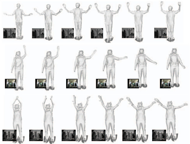
Figure 7. Results obtained with our method in different motion scenarios: a scenario with slow body and camera motion (1st row), a scenario with large frame-to-frame motion (2nd row), and a scenario with motion in topological change (3rd row).
