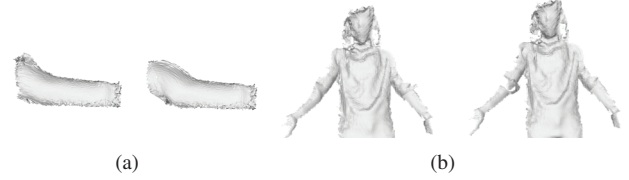
Figure 5. The comparison of the mesh with and without initial warping. (a) Final lower arm models in canonical space. The left one use the initial deformation in warp field, and the right doesn't; (b) final whole models in the last frame without fusion step.
