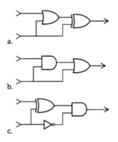
3. In each circuit below, the rectangles represent the same type of gate. Based on the input and output information given, identify whether the gate involved is an AND, OR, or XOR.
