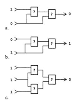
4. Assume that both of the inputs in the circuit below are 1. Describe what would happen if the upper input were temporarily changed to 0. Describe what would happen if the lower input were temporarily changed to 0. Redraw the circuit using NAND gates.
