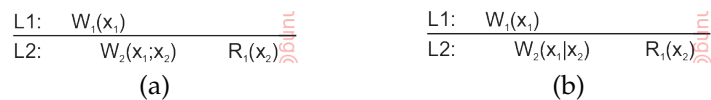
Figure 7.18: (a) A data store that provides read-your-writes consistency. (b) A data store that does not.
