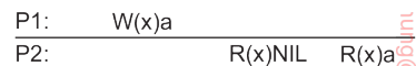
Figure 7.4: Behavior of two processes operating on the same data item. The horizontal axis is time.
