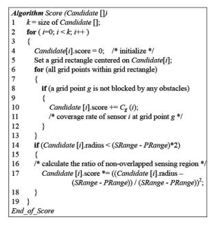
Fig. 10. Procedure of the Score algorithm.
