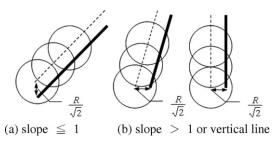
Fig. 6. Offset under different slope.
