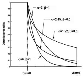
Fig. 3. The probabilistic sensor detection model.
