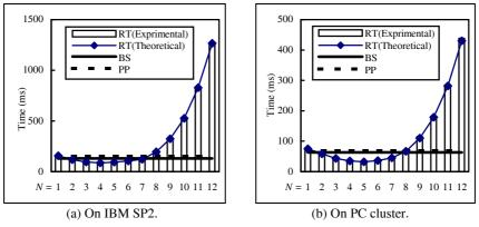
Fig. 9. The theoretical and experimental image compositing time of the BS, the PP, and the RT methods for test sample "*Engine*" with various numbers of initial blocks of a partial image.
