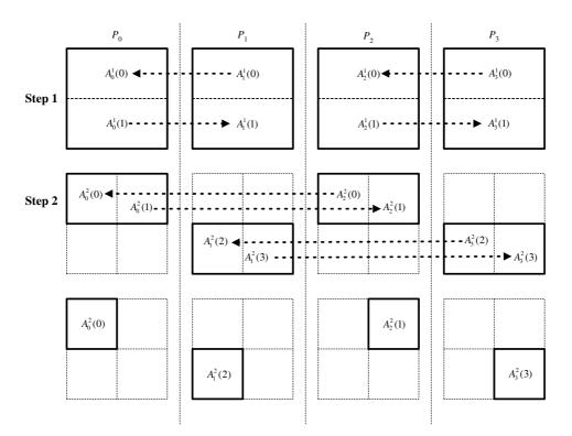
Fig. 1. An example of the BS method by using four processors.
