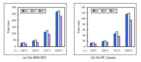
Fig. 14. The image compositing time of the BS, the PP, and the RT methods for test sample "Head" with various image sizes.
