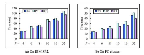
Fig. 11. The image compositing time of the BS, the PP, and the RT methods for test sample "*Head*" with various numbers of processors.
