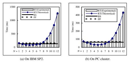
Fig. 7. The theoretical and experimental image compositing time of the BS, the PP, and the RT methods for test sample "*Bunny*" with various numbers of initial blocks of a partial image.
