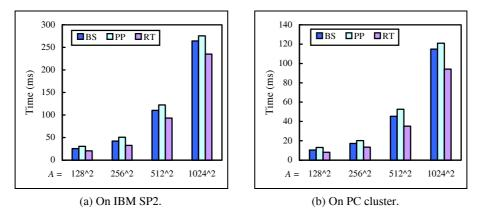
Fig. 15. The image compositing time of the BS, the PP, and the RT methods for test sample "*Engine*" with various image sizes.
