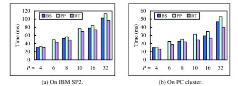
Fig. 10. The image compositing time of the BS, the PP, and the RT methods for test sample "Bunny" with various numbers of processors.
