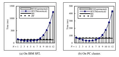
Fig. 8. The theoretical and experimental image compositing time of the BS, the PP, and the RT methods for test sample "*Head*" with various numbers of initial blocks of a partial image.
