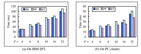
Fig. 12. The image compositing time of the BS, the PP, and the RT methods for test sample "*Engine*" with various numbers of processors.
