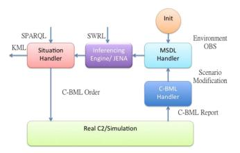
Fig. 12 Data flow of the Multi-layered Semantic Information Fusion Framework
