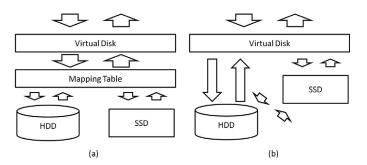
Fig. 1. The usage SSD in two scenario: Scenario (a) is the case which both SSD and HDD are combined into one virtual disk. The mapping table handle the re-direction of request. Scenario (b) is the case which SSD is the storage cache of HDD.
