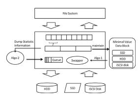
Fig. 3. The implementation of our heterogenous storage system management mechanism.
