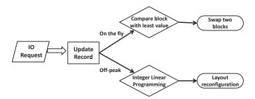
Fig. 2. The workflow of the trigger policy: When the new IO request coming, the system update the record and identify the request is hot or not. In the situation of on the fly, system only migration the block which value exceeds the threshold. In the situation of off-peak, the system will consider the full blocks and re-allocate into the suitable placement.
