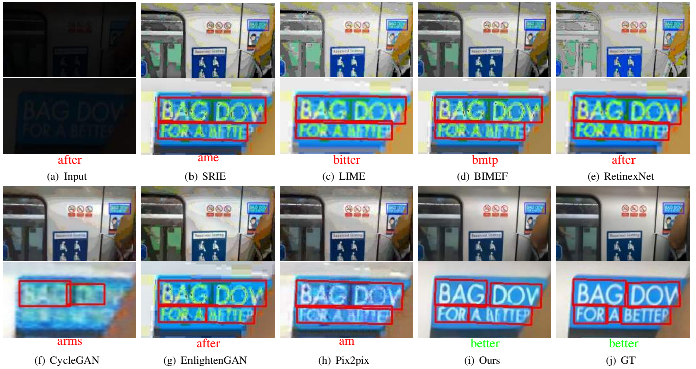
Fig. 4: CRAFT’s results (red boxes) of all methods on the ICDAR15 dataset, focused on the zoomed-in regions (blue boxes), followed by ASTER’s results based on the ground-truth bounding box of “BETTER”.
