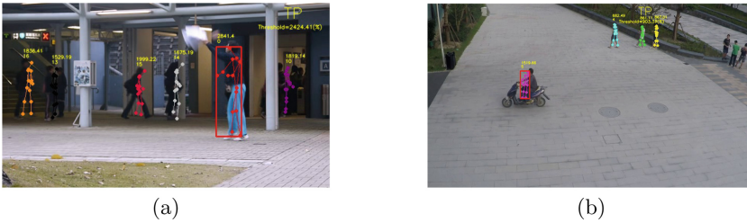
Fig. 4. Examples of the detected anomalies (in the red boxes). (a) In Avenue, the one unnaturally throwing the papers is detected since the model fails to reproduce his pose. (b) In ShanghaiTech, the one riding on the footway is detected since the model fails to adapt his speed. (Color figure online)
