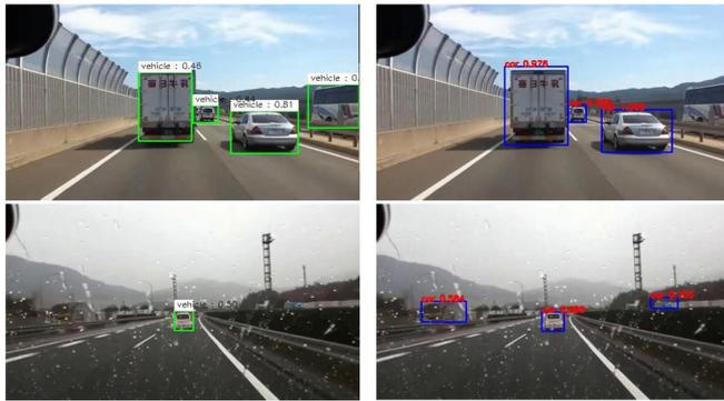
Fig. 11. iROADS selected detection results. Left column, detection results of this work (ResNet-50); Right column: detection result of Faster R-CNN (VGG-16); 1st row: Daylight; 2nd row: RainyDay.
