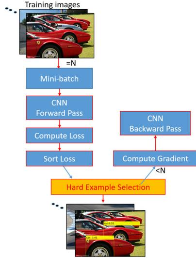
Fig. 4. The framework of OHEM applied to a single-stage detector.
