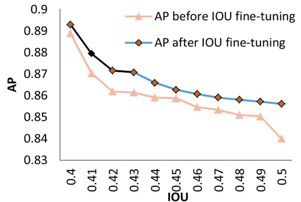
Fig. 15. AP corresponding to different IOU thresholds of our model (GoogLeNet) in VOC07 test.
