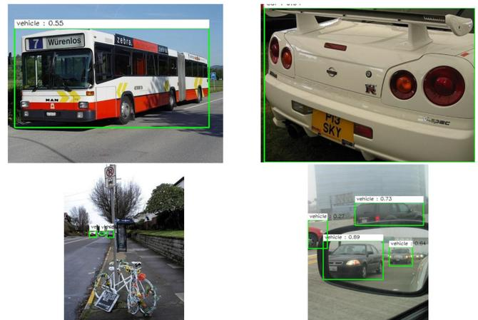
Fig. 7. Four typical scenarios of vehicle(s) expected to be detected. From top-left, top-right, bottom-left to bottom-right: one vehicle fully-seen, one vehicle partially-seen, small and fuzzy vehicles & occluded/truncated vehicles.
