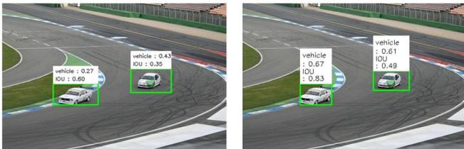
Fig. 14. Detection results before and after using bounding box priors. Left image: without priors. Right image: with priors.
