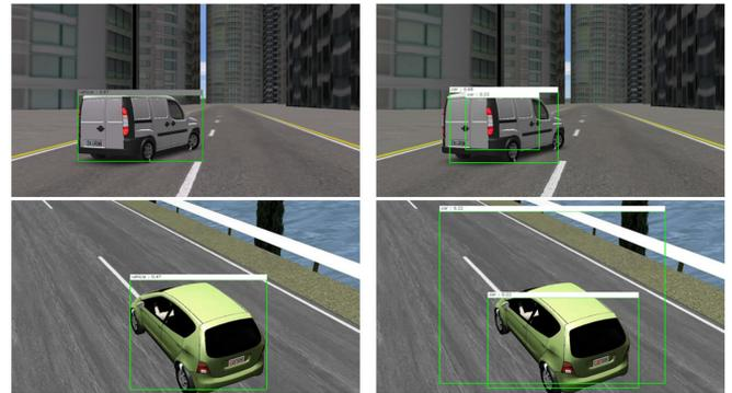
Fig. 10. Carsim detection result comparison; Left column: detection results of this work (ResNet-50); Right column: detection result of YOLO; 1st row: scenario-1 (vehicle-3); 2nd row: scenario-4 (vehicle-1).
