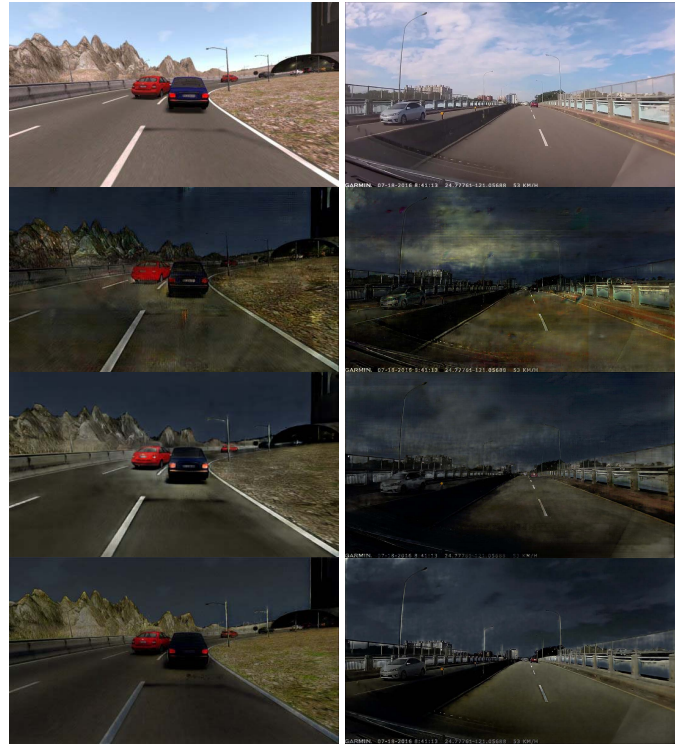
Fig. 12. SYNTHIA and ITRI-Day transformed results using AugGAN variations learning from SYNTHIA: left column: SYNTHIA input image and the transformed results using AugGAN-1, AugGAN-2, and AugGAN-3, respectively; right column: ITRI-Day input image and the transformed results using AugGAN-1, AugGAN-2, and AugGAN-3 learning from SYNTHIA, respectively.
