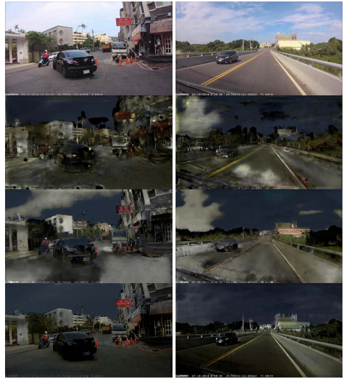
Fig. 6. ITRI-Day dataset day-to-night transformation results - GANs trained with SYNTHIA: 1st row: input images from ITRI-Day dataset; 2nd row: results of CycleGAN; 3rd row: results of UNIT; 4th row: results of AugGAN.
