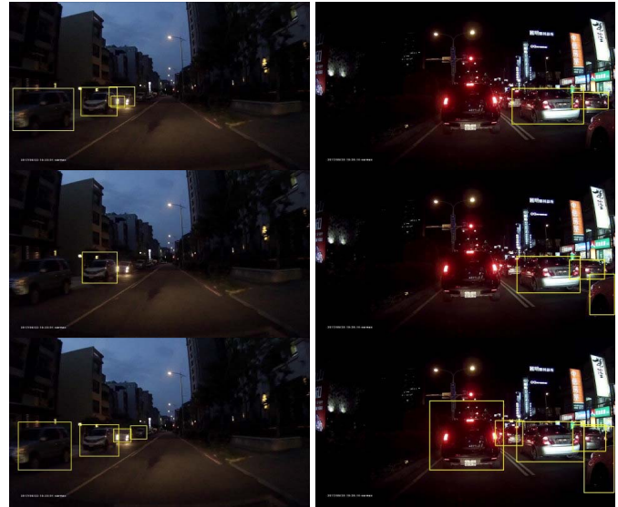
Fig. 10. Faster R-CNN detection result comparison: 1st row: ITRI-Night detection results using detector trained by KITTI-D2N-S (transformed by CycleGAN) training data; 2nd row: ITRI-Night detection results using detector trained by KITTI-D2N-S (transformed by UNIT) training data; 3rd row: ITRI-Night detection results using detector trained by KITTI-D2N-S (transformed by AugGAN) training data.
