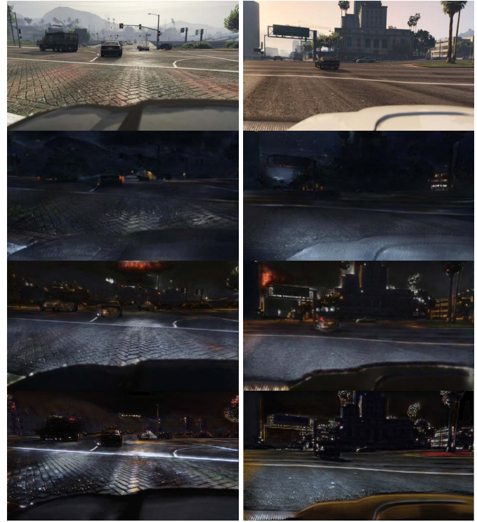
Fig. 3. GTA day-to-night transformation results - GANs trained with GTA: 1st row: GTA daytime testing images; 2nd row: results of CycleGAN; 3rd row: results of UNIT; 4th row: results of AugGAN.
