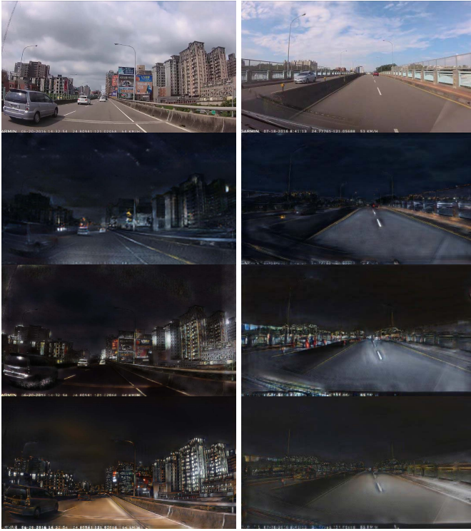
Fig. 7. ITRI-Day dataset day-to-night transformation results - GANs trained with GTA dataset: 1st row: input images from ITRI-Day dataset; 2nd row: results of CycleGAN; 3rd row: results of UNIT; 4th row: results of AugGAN.
