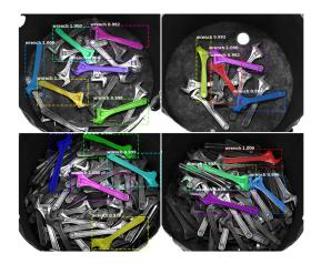
**Fig. 10**. Qualitative results on real data. Wrench detector is trained on both real and our synthetic data. Predicted results are shown in colored masks.
