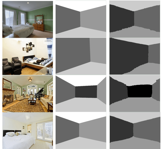
Fig. 7. Validation results under edge constraints and smoothness criterion in LSUN Room Layout. (Left) input image, (Middle) ground truth label, and (right) predicted layout. Note that the colors between ground truth and prediction are the same, labeling range is 1 to 5 and 0 to 4 respectively.
