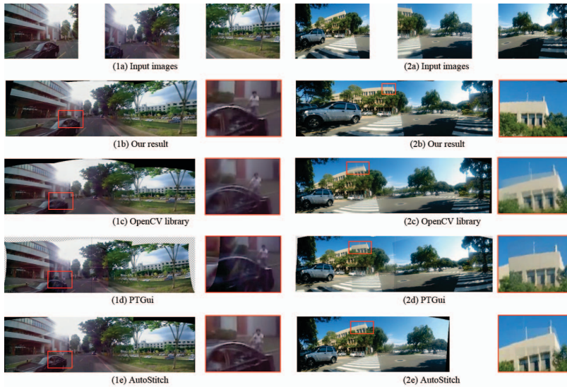
Fig. 5. We compare our results with openCV [2, 3, 9, 10, 11, 12], PTGui [13] and AutoStitch [14]. The second row shows our results from the input images (1a), (2a). We have better alignment than OpenCV (1c,2c), PTGui (1d,2d) and AutoStitch (1e,2e).
