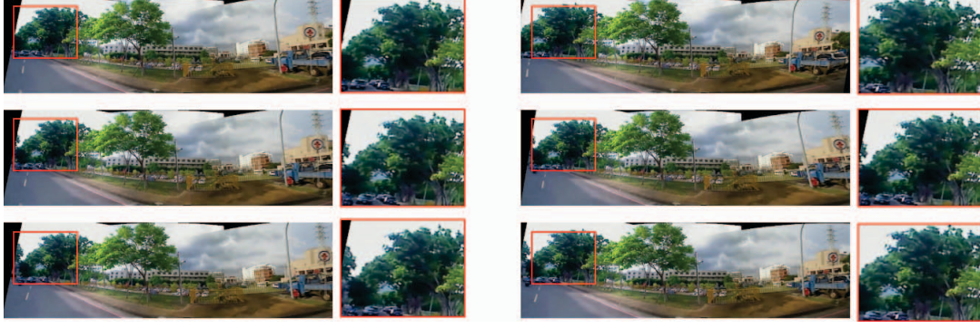
Fig. 4. Experimental results for video stitching with and without using temporal interpolation for homography estimation. The left column is with temporal interpolation while the right column is the result of homography estimation at every frame. Each column means 3 consecutive frames over time. The locations for the red blocks are fixed for all frames. The stitched images in the left column appear gradual changes along time, while the trees in the red blocks at the right column vary largely.
