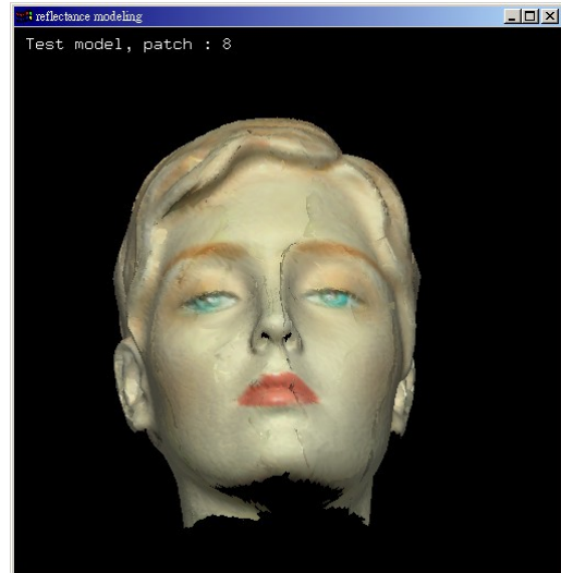
Figure 8: This is result of applying our reflectance modeling method. We blend the recovered ambient colors in the overlapped regions, and then illuminate the model under a new lighting condition.
